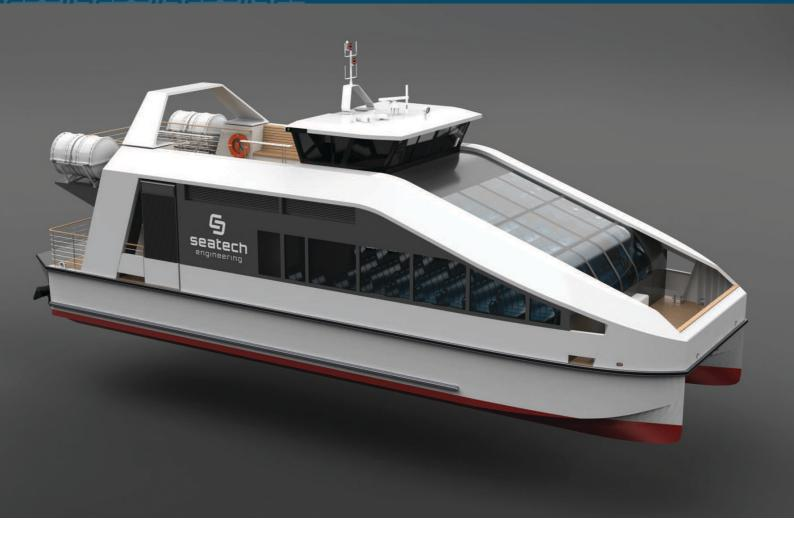
Inland Passenger Vessel 18 m Inland Passenger Vessel 18 m is designed by Seatech Engineering Ltd designing team. The main purpose of this project was creating a passenger catamaran for inland waterways. Following this assumption the vessel for most European river waterways should have draught and the overall high small applicably.
